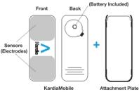
If you choose to attach KardiaMobile Hardware to the phone, adhere the optional attachment plate to the back of the phone.
